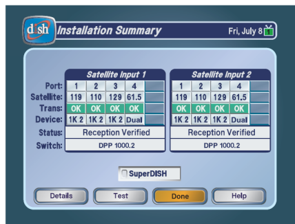
DISH Pro/DISH Pro Plus Installation Summary
